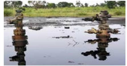
Fig. 8: Ogony Oil Spill showing damaged well head/BOP
